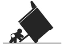
The range can tip forward, potentially causing injury and damage, if the anti-tip bracket is not properly installed. Do not operate the range without the anti-tip bracket in place.
