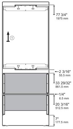
① This dimension line indicates the height measured from the floor.
