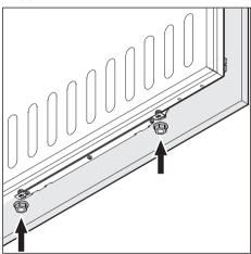
Screw the nuts onto the adjustment bolts and tighten them.
