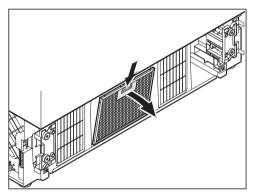
Push the latch of the air filter downwards and take it out.
