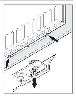
Tighten the adjustment bolts on the lower side of the appliance door until the mounting rail sits tight on the appliance door.
