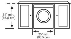
Minimum counter width should be 50" (127 cm) for a pair of Blomberg washer & dryer. Custom undercounter installation – Washer & Dryer
