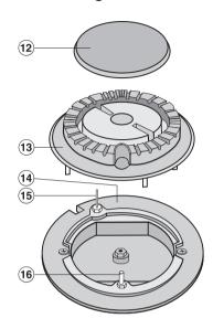
Be careful not to mix up the parts. Make sure that all the locating tabs and notches align exactly.
