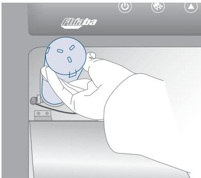
The filter is located inside the refrigerator compartment, above the top glass panel. Prior to changing the filter, switch off the Ice Maker by pressing the IceMaker button. Then enter the Fhiaba Access Menu and set "Manual Clean" function. At the end of the cleaning cycle remove the water from the ice tray and wipe it dry.
