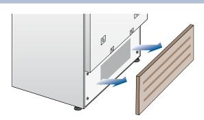
A ventilation grille is located either at the bottom of the appliance.
