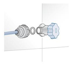
The models provided with Ice Maker require a connection to the domestic water supply system. This can be executed through the 1/4" water line (copper or polyethylene) to the house water supply. The system pressure must be between from 8 psi to 75 psi (between 0.5 bar and 5 bar).
