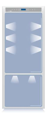
To provide optimum interior lighting, LED strips illuminate the refrigerator compartment from the top and sets of LED lights directly illuminate different areas of the refrigerator compartment, of the Crisper-Fresco drawers and the freezer drawer.
