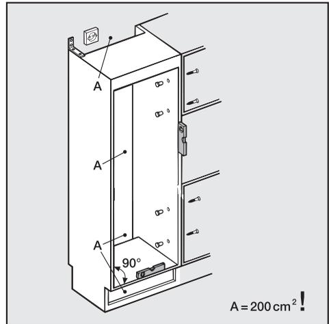
Before installing the appliance, the cabinetry must be carefully aligned using a level. The cabinetry corners have to be 90° angles, otherwise the cabinetry door will not be flush with all 4 corners of the cabinetry.
