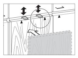
**Tip:** Slide the fitting aids (2) and the cabinet front up to the height of the adjacent cabinet unit doors.
