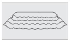
Lift the front of the rack and slightly pull the rack forwards until the notch at the side is in line with the shelf support. The rack can then be raised or lowered to the desired level.
