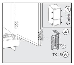
Screw the mounting bracket ④ onto the pre-drilled holes in the appliance door using the hex screw ⑤.
