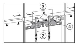
Remove the nuts ③ and detach the mounting frame ④ together with the fitting aids ②. Lay the cabinet door face down on a stable surface.
