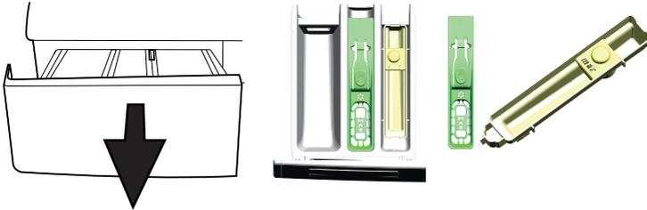
1. Press the dotted point on the siphon of the softener compartment and pull towards yourself until the it is removed from the dispenser.
