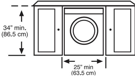
Minimum counter width should be 50" (127 cm) for a pair of Blomberg washer & dryer.
