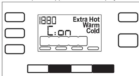
The same symbol will also be displayed whenever any button is pressed while the washer is child-locked.
