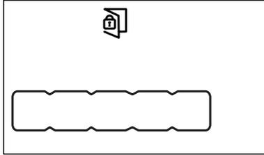
When the electricity is off in door locked position, door will keep the locked position for two minutes. After two minutes, door is allowed to open.
