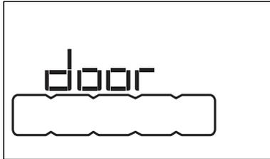
In case the door is not locked, "door" expression will appear on the screen. In that case, door should be opened and closed again firmly.
