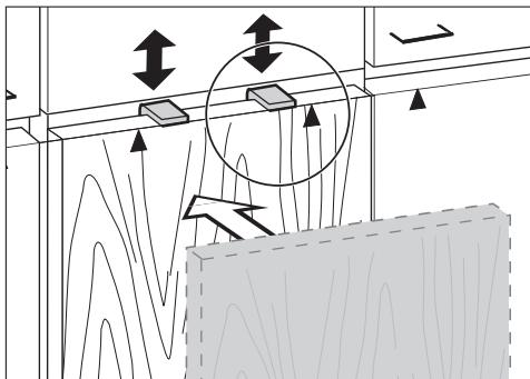
**Tip:** Push installation aids ② to the height of the adjacent cabinet doors with the cabinet front.
