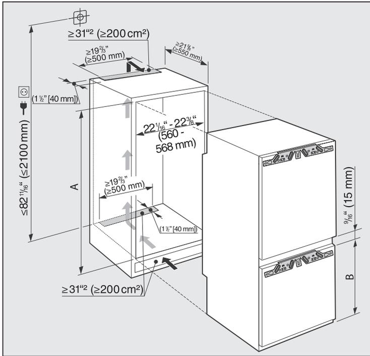
\* The declared energy consumption was achieved with a niche depth of  $22 \frac{1}{16}'' (560 \text{ mm})$ . The appliance is fully capable of functioning at a niche depth of  $21 \frac{5}{8}'' (550 \text{ mm})$ , but will consume slightly more energy.
