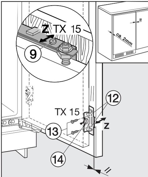
■ Pre-drill fixing holes ⑫ in the cabinet door and fasten screws ⑬. Make sure both metal edges are flush (// symbol).
