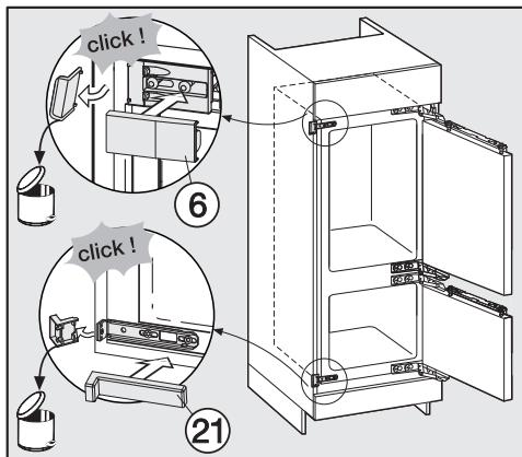
To give the appliance additional security in the niche push the batons supplied between the appliance and the cabinet base:
