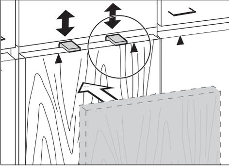
**Tip:** Push installation aids ② to the height of the adjacent cabinet doors with the cabinet front.
