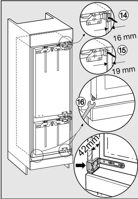
■ Now push the appliance into the niche until all securing brackets make contact with the front edge of the cabinet side wall.
