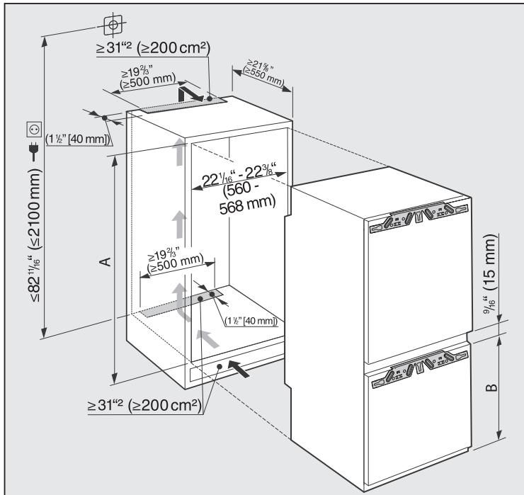
\* The declared energy consumption was achieved with a niche depth of 22 1/16" (560 mm). The appliance is fully capable of functioning at a niche depth of 21 5/8" (550 mm), but will consume slightly more energy.
