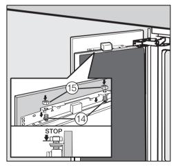
Open the door and hang the custom door with the mounting frame over the threaded bolts <sup>(4)</sup>.
