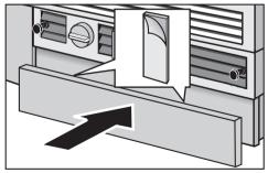
Remove the foil from the adhesive strips.
