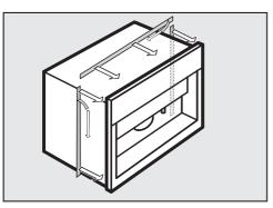
■ If the housing unit niche is not fitted with a sealing strip, you should fit a Miele sealing strip to the machine before installing it. This is fitted from the back of the machine
