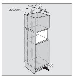
Air intake ① occurs via the plinth at the bottom of the machine and the air escapes at the top ② at the rear of the housing unit.
