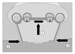
■ To remove the sensor cover, press and hold the cover ① between the two dispensing spouts. Then press the sides of the central spout ② at the back.
