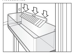
Attach the bottle holder centrally along the rear edge of the bottle shelf, as shown. The flexible ribs on the holder grip the bottles securely when the door is being opened and closed.
