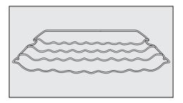
Bottles can be stored horizontally using the bottle rack to save space. The bottle rack can be placed at different positions in the appliance.
