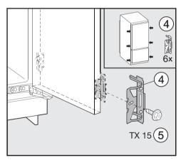
■ Screw fixing bracket ④ using hex screw ⑤ to the pre-drilled holes in the appliance door. Using the pre-drilled holes in the appliance door, secure a second pair of fixing brackets ④ in the handle area of the door.
