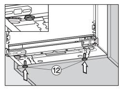
■ Screw in adjustable feet ② completely.
