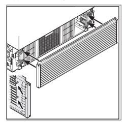
Now install the base cover with the ventilation slits. There are two fastening bolts on each side of the base cover (see illustration detail). These fastening bolts must be inserted into the retainer holes.
