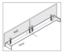
Securing to a wooden floor (screws: 1/4" x 2 1/2") (6 x 63 mm)
