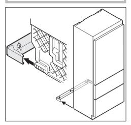
Gently push the appliance into the niche until the back of the appliance slides into the anti-tip bracket.
