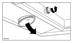
Turn the bolt counterclockwise as far as it will go. The halogen lamp will then drop down towards you.
