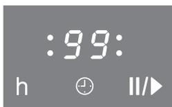
In case of a time of more than 99 minutes, the timer must be switched to hours (h). The time is set in half-hour steps. Half-hours are indicated by a dot following the number, for example, 2 h 30 min:
