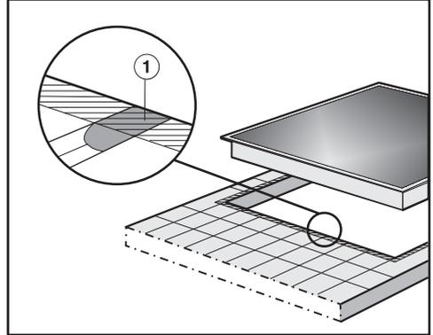
The grouting ① and the shaded area under the cooktop frame must be smooth and flat so that the frame will sit evenly on the countertop and so that the sealing strip under the top edge of the appliance can provide an adequate seal with the countertop.
