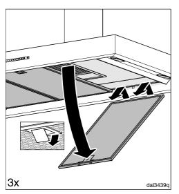
■ Remove the grease filters from the cooker hood.
