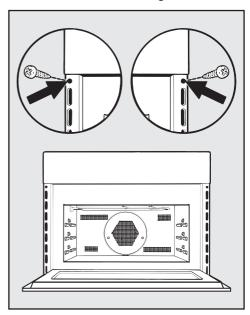
■ Open the door and use the screws supplied to secure the oven to the side walls of the cabinetry through the holes in the oven trim.
