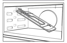
Carefully lower the Browning / Broiling element. The cover at the top of the oven cavity can be damaged.
