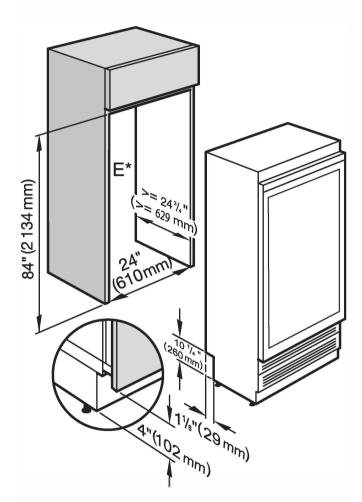
$\mathsf{E}^*:$  The position of the electrical connection should not be higher than 9" from the floor.
