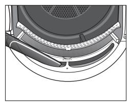
Use a vacuum cleaner with a long crevice nozzle attached to remove any visible lint from the upper air flow openings.
