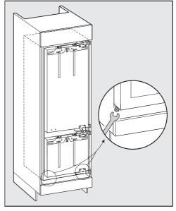
Align the appliance on both sides via the adjustable feet so that it stands level.
