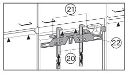
Unscrew the nuts ② and remove the mounting frame ② together with the installation aids ②. Place the cabinet door on a stable surface with the outer side facing downward.
