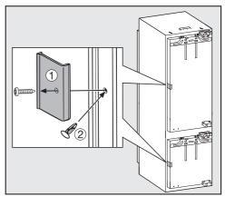
■ Remove red transport safety device ① (depending on model) and use the stopper supplied to cover the hole ②.
