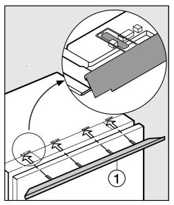
■ Push the filler strip lugs ① into the holders from the front.
