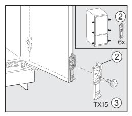
■ Loosely screw the securing brackets ② into the pre-drilled holes in the appliance door using hex screws ③.
