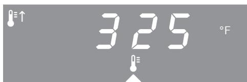
The altered target temperature is saved. The actual temperature is displayed.
