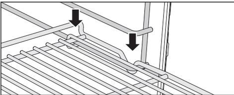
Always place the wire oven rack on the runner with the notch facing down.
