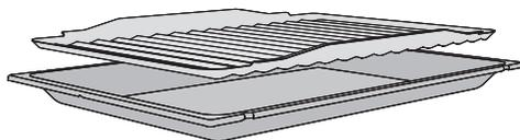
Use the universal tray with the grilling and roasting insert (if available), and place the tray in the oven. The insert prevents any collected meat juices from burning, allowing them to be used for gravy and sauces.
