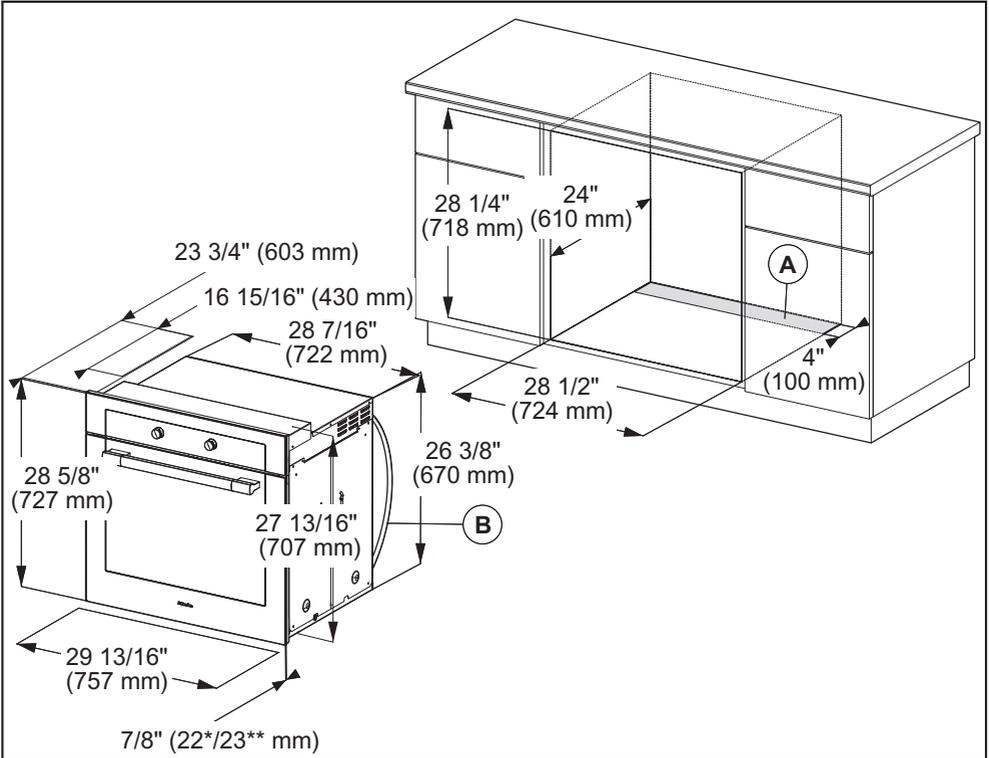
Ⓐ Cut-out ( $4 \times 28 \frac{3}{8}$ " /  $100 \text{ mm} \times 720 \text{ mm}$ ) in the bottom of the cabinet for power cord and ventilation
