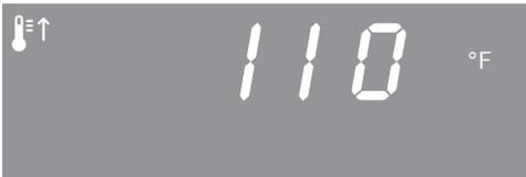
You will see the temperature rising in the display. A buzzer will sound when the oven temperature is reached if this option is selected (see “Settings -  $\frac{E1}{7B} 2$ ”).
