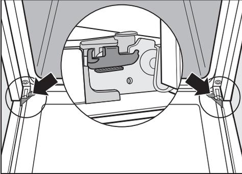
The oven door is connected to the hinges by retainers. Before removing the door from the retainers, the locking clamps on both hinges have to be released.
