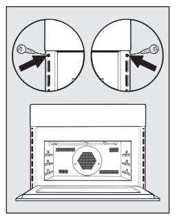
Open the door and use the screws supplied to secure the oven to the side walls of the cabinetry through the holes in the oven trim. Please have the model and serial number of your appliance available when contacting Customer Service.
