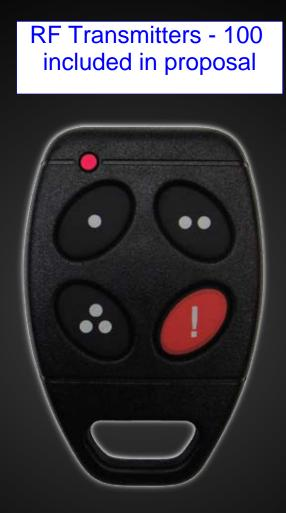
The Wireless 433MHz 4 Button Transmitter is designed for long range wireless access control of garage doors or sliding gates. Each transmitter is encoded with a 'Wiegand' compatible ID number so that usage can be controlled and recorded by most electronic access control systems on the market.
