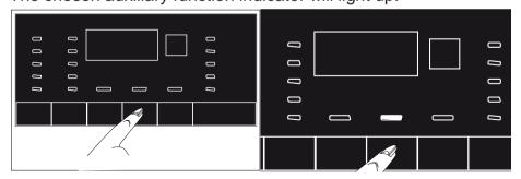
Furthermore, you may also select or cancel auxiliary functions that are suitable to the running programme without pressing the Start / Pause button when the machine is operating. For this, the machine must be in a step before the auxiliary function you are going to select or cancel.
