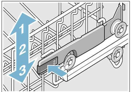
**Note:** Check spray arm for clearance after adjustment.
