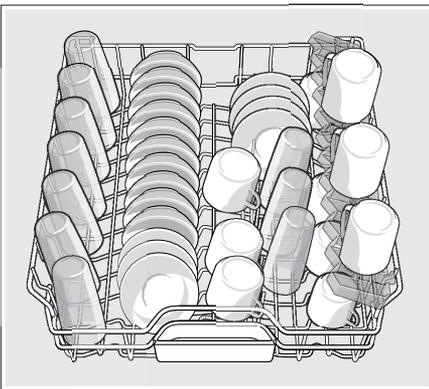
**Note:** Folding the cup shelves down will allow the cups to sit at an increased angle and reduce water pooling on cup bottoms.
