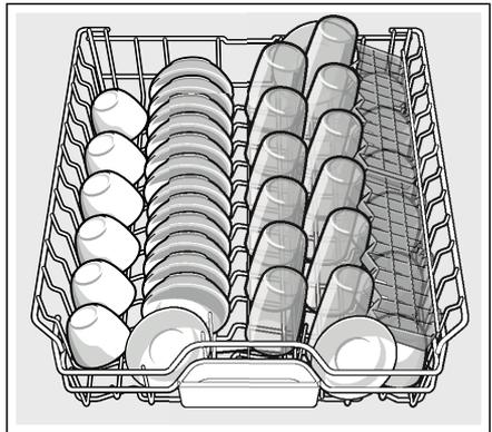
**Note:** Folding the cup shelves down will allow the cups to sit at an increased angle and reduce water pooling on cup bottoms.
