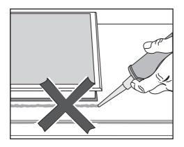
Using sealant under the cooktop could result in damage to the cooktop and the countertop if the cooktop ever needs to be removed for servicing.
