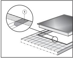
Grout lines ① and the shaded area under the cooktop frame must be smooth and even. If they are not, the cooktop will not sit flush with the countertop and the sealing strip underneath the cooktop will not provide a good seal between the cooktop and the countertop.
