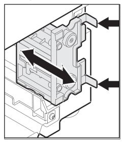
The face end of the angles on the retainers must be flush with the front of the toe-kick cover. If this is not the case, adjust the retainers according to the depth.
