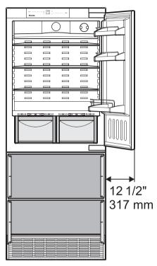
These measurements do not take the cabinet front and the door handle into account; they must be added on accordingly.
