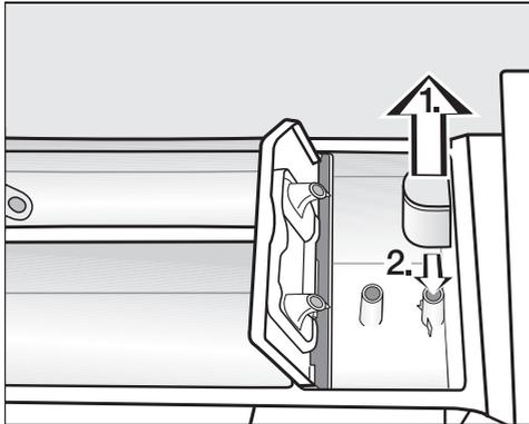
1. Remove the siphon from the ☸ compartment and clean under warm running water. Clean the siphon tube in the same way.
