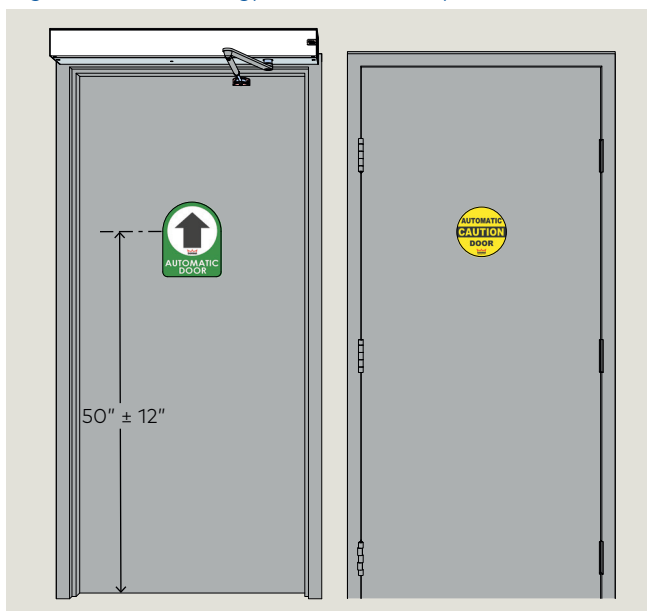
Fig. 7.3.2 Full energy decals, two way traffic
